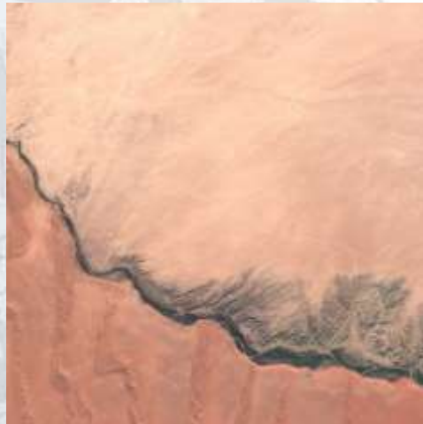
Gobabeb , in Namibia. Large Hyper-arid desert with minimal vegetation and stable atmospheric conditions. Ideal for radiometric calibration due to its consistent surface and low humidity
