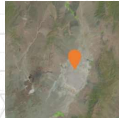
Railroad Valley Playa, USA. Large, flat playa (dry lakebed) with consistent reflectance properties. Used for radiometric calibration of sensors: Landsat and MODIS instruments.
